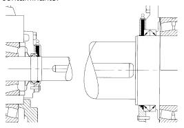
To remain effective, the protective grease must be purged periodically. The regreasing schedule should be based on the severity of the operational and environmental conditions. In severe conditions the regreasing should be performed every 1 to 2 months. Under more favorable conditions regreasing schedule could be extended to 3 to 6 months.
