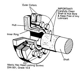
LOCKING SCREW-TIGHTENING TORQUES "MA"
