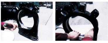
Remove the old EPDM seal ring, clean the body space of the seal ring and mount a new EPDM ring
