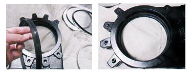
Re-assemble the retainer on the EPDM seal ring, hammering gently around the edge,
